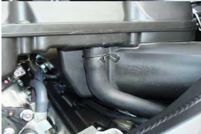
Fig. 2. REINSTALL HOSE OVER PLUGGED PORT
