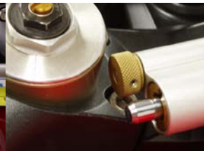
Inspect clearance steering must be unobstructed from stop to stop!
