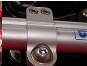
Torque 8MM to: (17.2N•m/13 ft•lb.) (Figure 7)
