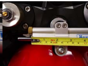
Adjust position (@ 1.75 in./44.5mm) Torque 5MM clamp bolts (3.4N•m/30in•lb.)
