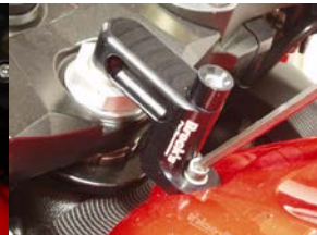
Torque to: (12N•m/106in•lb.) (Figure 3)
