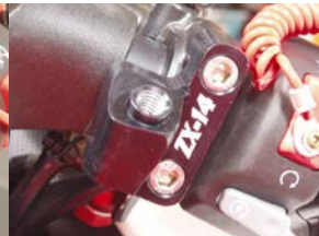
Torque both screws (8.8N•m/106in•lb.) (Figure 4/5)
