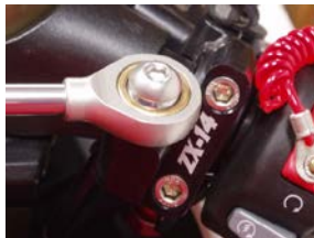
Torque 8MM to: (17.2N•m/13 ft•lb.) (Figure 6)
