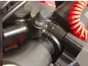
Install master cylinder bracket- reassemble at dimple on top of the stock clamp
