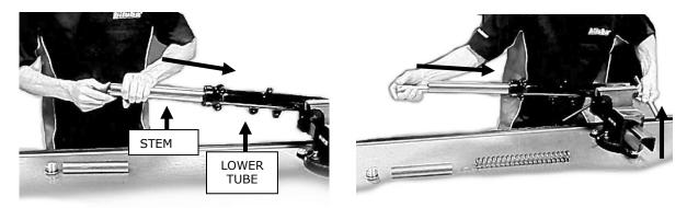
13. Holding the stem at the bottom of the lower tube, take the original piston out with the original top out.
