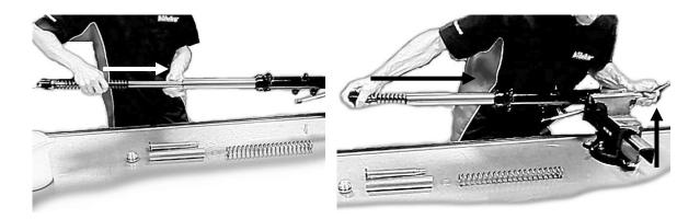
17. Position the cartridge vertically. Pour Bitubo oil code 997630, for the quantity refer to the table "1" in the BASIC SET-UP section (pag. 1). Perform some compressions and extensions of the fork tube to allow the oil to load correctly.
