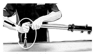
7. Remove the original spring and shims.
