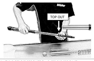
16. Holding the stem on the bottom of the lower tube, insert the BITUBO cartridge into the fork and fix it with the original Allen screw and washer, tightening correctly to the torque stated by the manufacturer.
