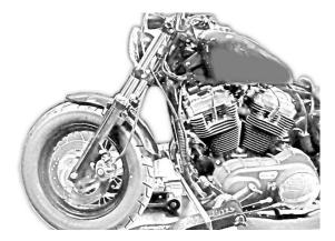
2. Remove the wheel and all the devices connected to the fork following the instructions in the user's manual of the original vehicle.
