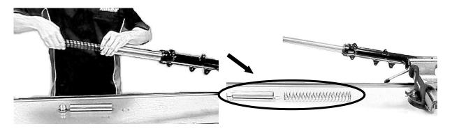
8. Overturn the fork leg and empty the oil from the lower tube.
