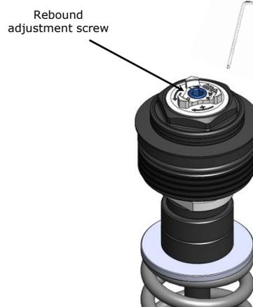
Both adjustments can be performed with a common male hex key with a 4mm spherical head.
