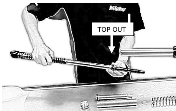
13. Holding the stem on the bottom of the lower tube, insert the BITUBO cartridge into the fork and fix it with the original Allen screw and washer, tightening correctly to the torque stated by the manufacturer.
