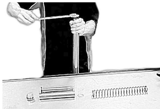
17. Make hydraulic adjustments and spring preload before installing the fork leg on the bike. The limited space between the handlebar and upper caps does not facilitate access to settings.
