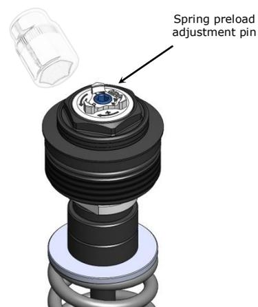
The adjustment of the spring preload can be made with a common 17mm hexagonal bushing.
