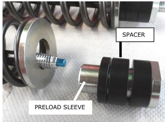
4. According to the selected length reduction, remove the number of shims shown in the table.
