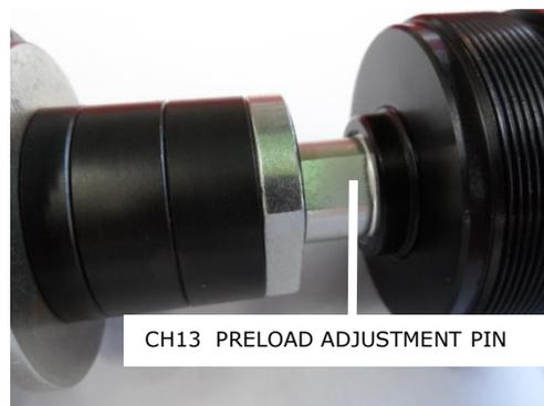
2. Loosen and unscrew the cap holding the 13mm key of the preload adjustment pin and the 22mm key of the preload sleeve.
