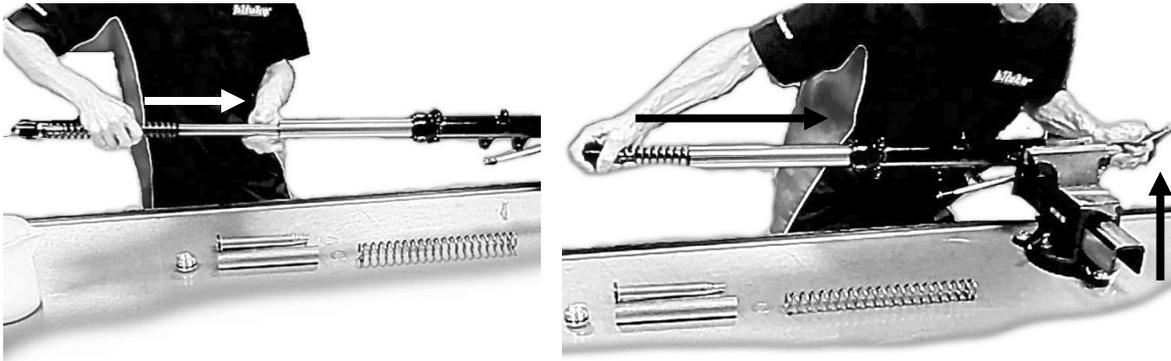
14. Position the cartridge vertically. Pour Bitubo oil code 997630, for the quantity refer to the table "1" in the BASE SET-UP section (pag.1). Perform some compressions and extensions of the fork tube to allow the oil to load correctly.
