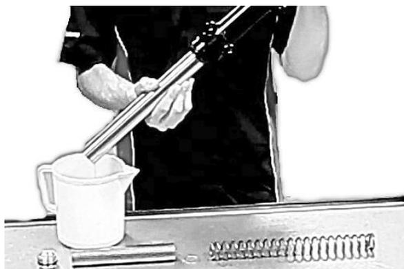
9. We recommend you check the fork stem and lower tube slide correctly without any friction and do not seize.
