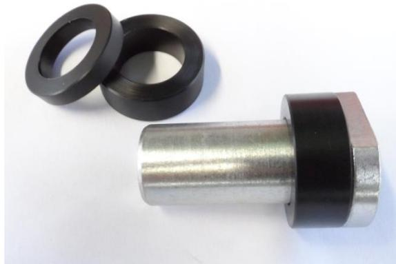
5. Refit the preload sleeve and any remaining shims.
