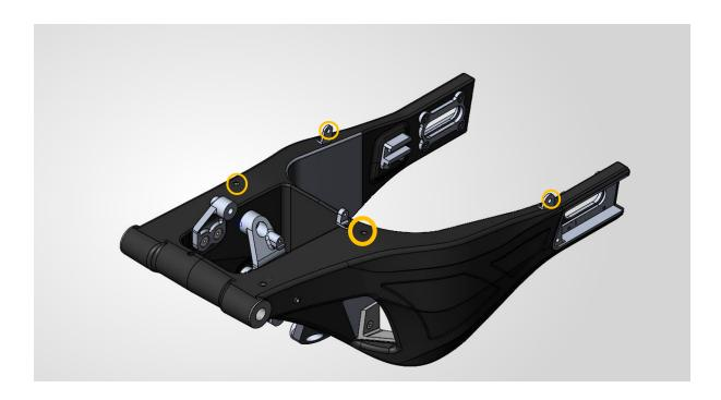
The final screw holding the chain guard to the swingarm is an M5 Hex screw near the strut mount, remove and keep the M5 screw.
