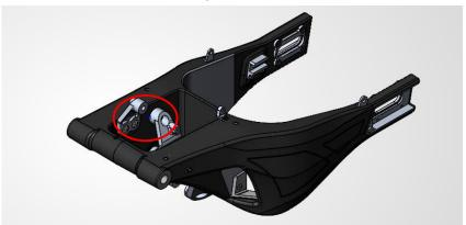
4. Align the shock assembly with the bottom shock mount and torque to OEM specifications.
