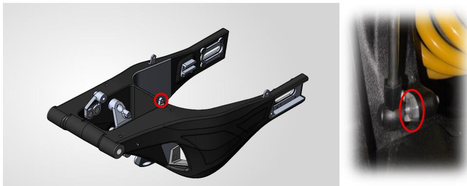
6. Remove the screw that secures the suspension strut (to be used on the Carbon Swingarm)
