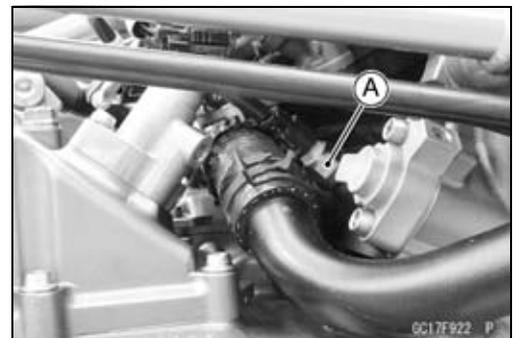
Gear Position Sensor [A]
