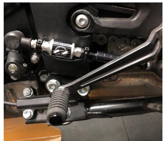
**Fig3. Rod & Sensor Install**
