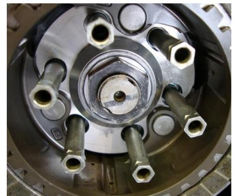
**Attention: Although casual riding is generally unaffected after the installation of the Clutch Mod, some rear wheel "chirp, hop, or chatter" may be noticed.**
