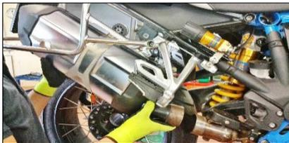
**ENG** Unscrew the screw of the silencer support bracket and remove the original exhaust.
