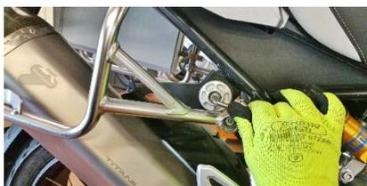
**ENG** Tighten all the screws starting from the one of the silencer support bracket, then the bracket fixing screw to the frame and at the end the small metal bracket placing it as shown in the picture.
