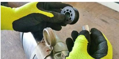
**ENG** Remove the original rubber and spacer, keep them for mounting the Termignoni kit
