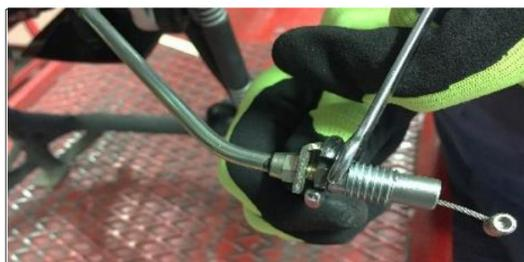
**ENG** Insert the cable in the seat and screw the adjuster body at the end of its stroke, tighten with a wrench 8 mm for the adjuster body and with a wrench 10 mm for the nut on the cable.
