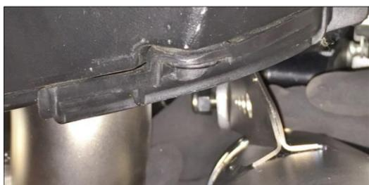
**ENG** Screw the silencer support bracket to the connecting rod using the washer and screw supplied placing them in front of the bracket and using the washer and the nut placing them in the back of the bracket
