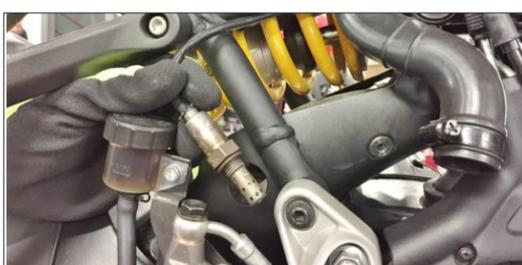
**ENG** Unscrew and remove the lambda probe
