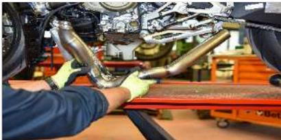
*Insert the horizontal collector pipe (5) and place the 4 springs (15). Insert the 2 caps (45) with copper washers (40) on the collectors. Alternatively, it is possible to use the standard probes with the caps (46) and copper washers (40) and (44)*
