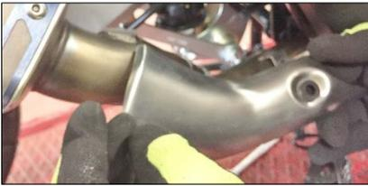
**ENG** Remove the original heat shield unscrewing the support screw
