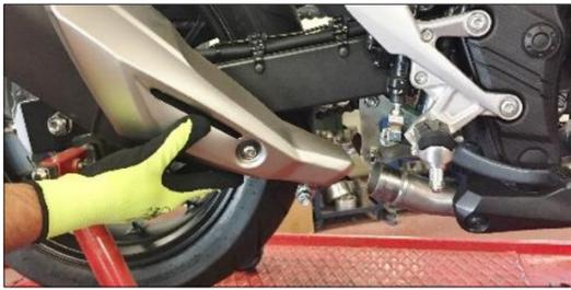
**ENG** Unscrew the screw of the silencer support bracket and remove original exhaust.
