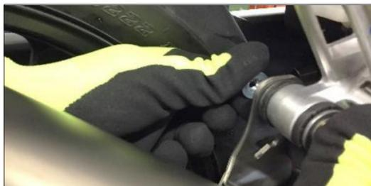
**ENG** Fix the support bracket to the silencer, using the original screw, washer and nut without tightening
