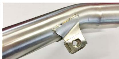
**ENG** Position the clip M8 on the silencer, right and left, support bracket
