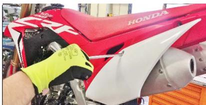
**ENG** Unscrew the fixing screws to the seat and to the side panels right and left side
