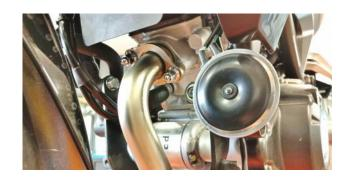
**ENG** Mount the Termignoni collector, inserting the bush and flange (head attacks) in its housing, fixing it with the original nuts without tightening.
