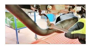
**ITA** Svitare la sonda lambda. **ENG** Unscrew the lambda probe.
