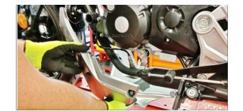
**ENG** Unscrew the belly pan support screws, then remove it.
