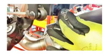
**ENG** Fix the silencer to the frame using the original screw previously removed and the nut in the pack, whithout tightening.
