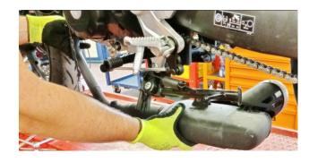
**ENG** Unscrew the screw of the silencer support bracket and keep it fot the mounting of the Termignoni silencer and remove original exhaust.
