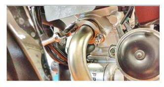
**ENG** Tighten all the screws starting from the one of the silencer support bracket. Screw and lock probe
