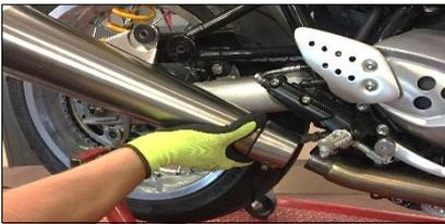
**ENG** Unscrew the screws to small metal clamp and and remove original exhaust
