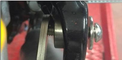
**ENG** Fix the bracket to the frame using the screw M8x35, the washer M8x24 and spacer in the pack, placing them as in the picture, without tightening
