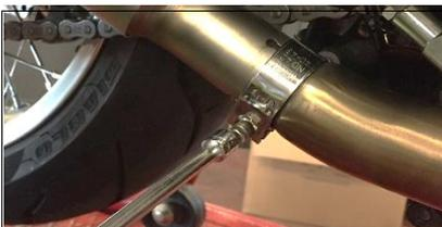
**ENG** Tighten all screws starting from the one of the bracket fixing screw on frame and at the end the small metal bracket.
