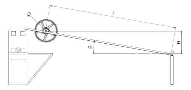
Fig. 02 Rotational Inertia Test Rig
