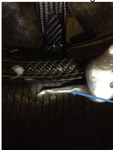
Figure 5: 5 mm radial gap between the rim and the foot
